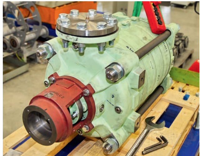
Fig. 2: Prototype of a liquefied gas pump
