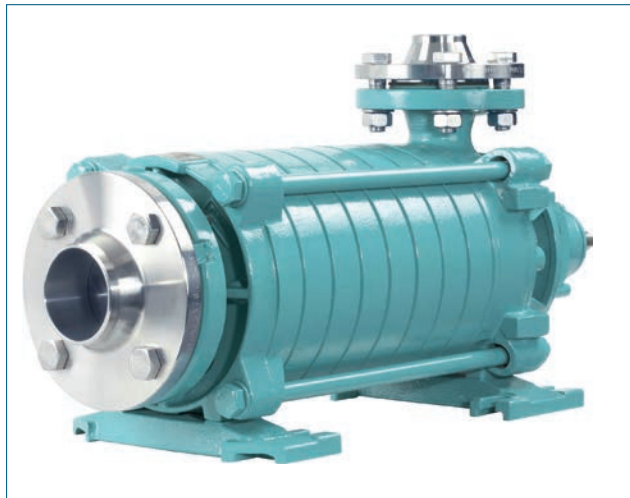
Fig. 1: Liquefied gas pumps achieve a flow rate of up to 340 m 3 /h with a pressure of up to 40 bars and a temperature range from -40 °C up to 110 °C. The viscosity can be up to 115 mm 2 /s.
