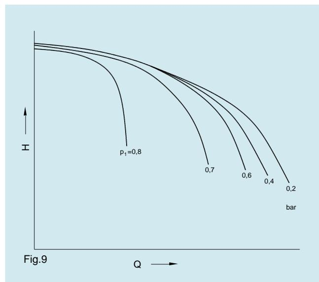
Only this range is free of cavitation being in congruence with that throttle curve being assigned to a smaller vacuum. It shows that the cavitation-free working range of a pump is getting smaller the higher the vacuum is. In case of very high vacuums no further contact exists to other curves, i.e. at each rate of flow the pump operates with cavitation.
