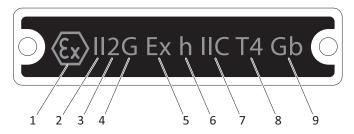
Fig. 1-3 ATEX type plate on the pump casing
