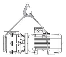
Fig. 5-1 Transporting the pump with a crane
