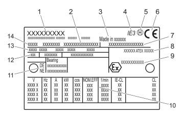
Fig. 1-4 Type plate on the motor
