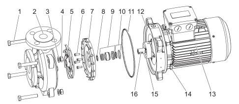
Fig. 10-4 Removing the shaft seal, example
