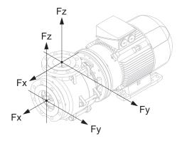
Fig. 7-2 Permissible forces and torques
