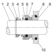
Fig. 10-6 Design of the mechanical seal with conical spring
