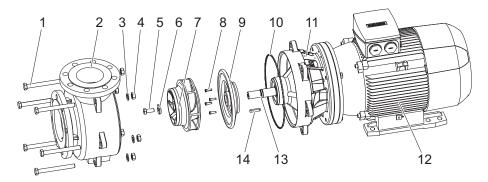
Fig. 10-7 Installing the casing, example
