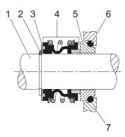
Fig. 10-5 Design of mechanical seal with elastomer bellows and O-ring
