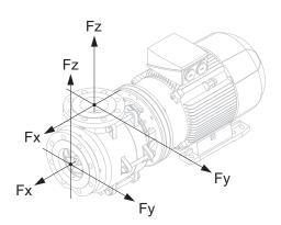
*Fig. 7-2 Permissible forces and torques*
