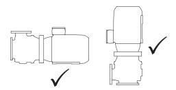
Fig. 7-1 Permissible installation positions
