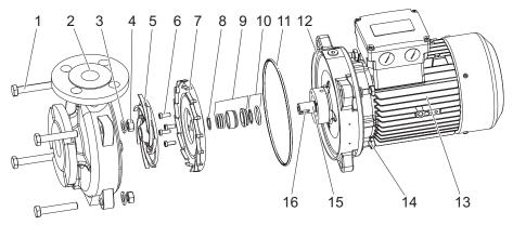
Fig. 10-4 Removing the shaft seal, example
