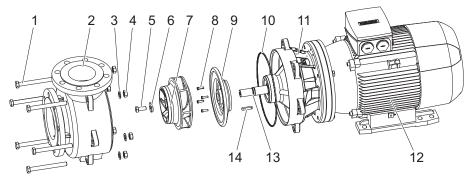
*Fig. 10-7 Installing the casing, example*
