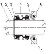
*Fig.* 10-5 *Design of the mechanical seal with elastomer bellows and o-ring*
