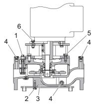
Fig. 10-2 LUBLS tightening torques
