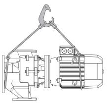
Fig. 5-1 Transporting the pump with a crane
