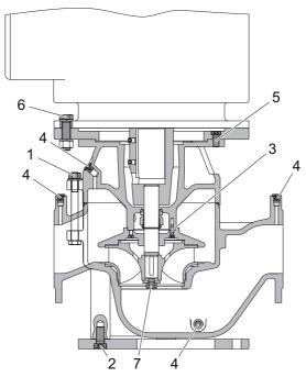
Fig. 10-3 LUBS tightening torques
