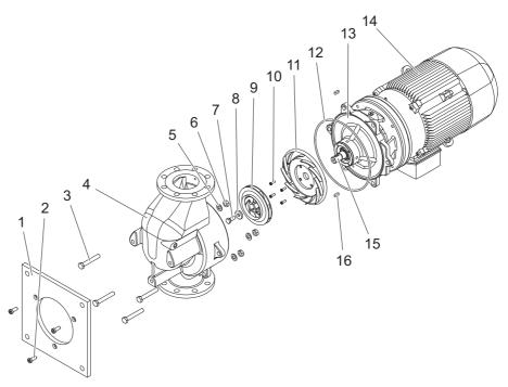
*Fig.* 10-7 *Installing the casing, example*
