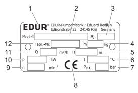
Fig. 1-2 Type plate on the pump casing
