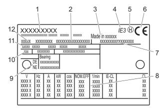
*Fig. 1-3 Type plate on the motor*
