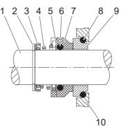
Fig. 10-6 Design of the mechanical seal with conical spring
