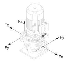
Fig. 7-2 Permissible forces and torques
