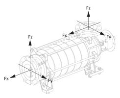
Fig. 7-2 Permissible forces and torques
