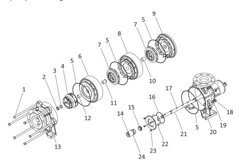
Fig. 10-4 Removing the shaft seal, example
