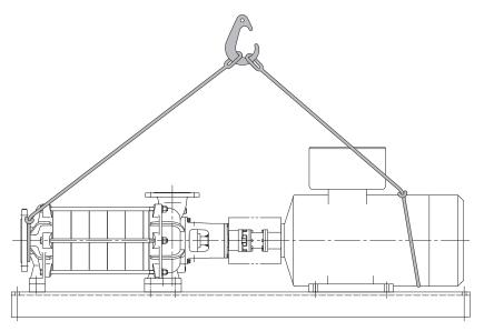
Fig. 5-2 Pump with motor mounted on a base plate
