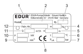
Fig. 1-2 Type plate on the pump casing
