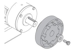
Fig. 7-6 Pump shaft and pump-side half of the coupling
