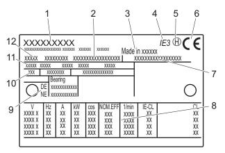
Fig. 1-3 Type plate on the motor
