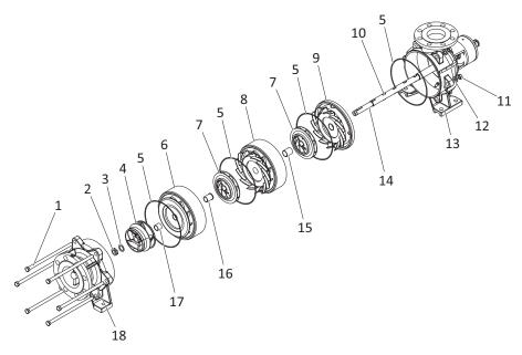
Fig. 10-7 Installing the casing, example
