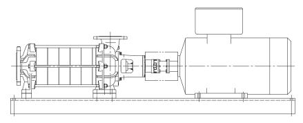
Fig. 4-6 Expansion stage A, pump coupled to motor, mounted on base plate, with coupling guard
