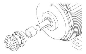
Fig. 7-7 Motor-side coupling half (unit consisting of half of coupling, spacer and cam ring) and spacer sleeve
