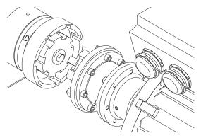
Fig. 7-8 Pump-side and motor-side halves of the coupling
