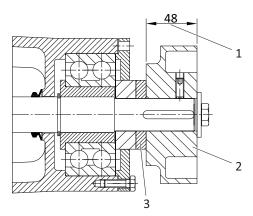
Fig. 7-4 Example for assembly of the coupling hub with spacer washer
