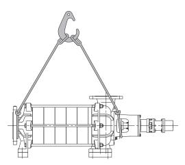
Fig. 5-1 Pump without motor and not mounted on a base plate
