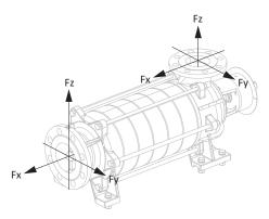
Fig. 7-2 Permissible forces and torques
