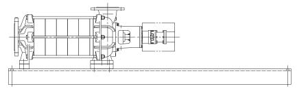
Fig. 4-5 Expansion stage G, pump with coupling, mounted on base plate, with coupling guard
