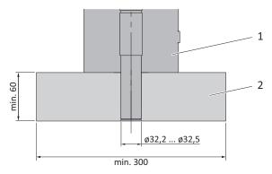
Fig. 10-2 Auxiliary structure for vertical removal and fitting
