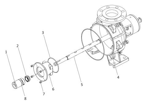
Fig. 10-6 Installing the relieved mechanical seal
