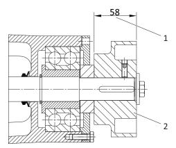
Fig. 7-3 Example for assembly of the coupling hub
