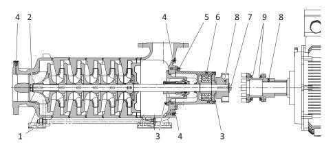
Fig. 10-1 Tightening torques NHE/NHKE
