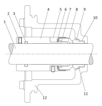
Fig. 10-5 Design of the relieved mechanical seal with sinusoidal spring
