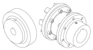
Fig. 7-5 Pump-side and motor-side halves of the coupling with spacer and cam ring
