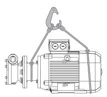
Fig. 5-1 Transporting the pump with a crane
