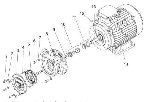
Fig. 10-3 Removing the shaft seal, example
