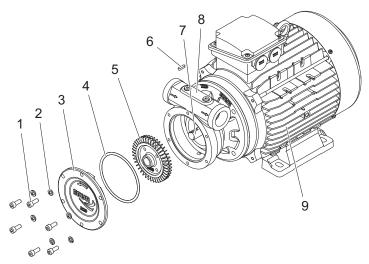
Fig. 10-6 Installing the cover, example
