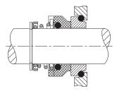
Fig. 4-2 Design of mechanical seal with conical spring
