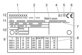
Fig. 1-3 Type plate on the motor
