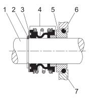
Fig. 10-4 Design of the mechanical seal with elastomer bellows and o-ring
